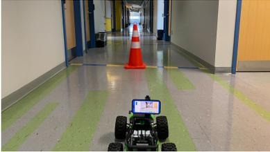
Fig. 5. An obstacle from the training obstacle set is set seven feet from the vehicle.
